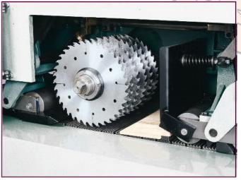
The saw arbor is manufactured from Ni-Cr-Mo alloy steel, heat treated, precision grinding, and dynamically balanced for maximum durability and stability.
