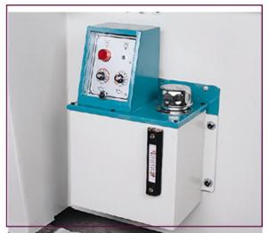
The automatic lubricator offers frequent lubrication between the caterpillar chain and rail.
