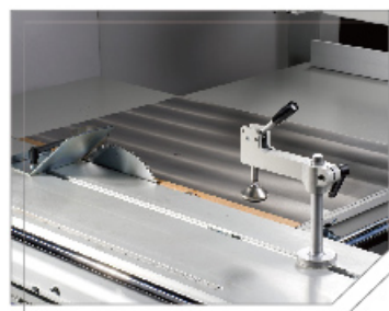
Rapid Clamp (Right Side) Clamp Shoe (Left Side)
